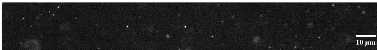
Fig. 5 Dark-field microscopy image of the Janus nanoparticles. A representative frame acquired during the experiments (see Movie S1 in the SI), showing Janus nanoparticles in the absence of optical excitation. Although individual nanoparticles are subject to optical resolution limits, this does not prevent the precise determination of their center-of-mass position via single particle tracking (see Material and methods). The sample concentration is set in the dilute regime at c \approx 3.6 \times 10^9 particles per mL.
