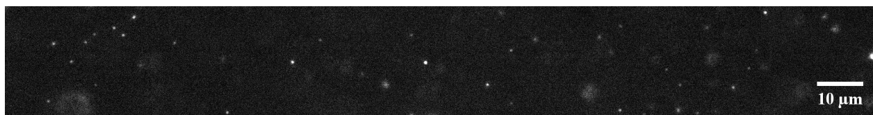
Figure 5: Dark-field microscopy image of the Janus nanoparticles. A representative frame acquired during the experiments (see Supplementary Movie S1 in the SI), showing Janus nanoparticles in the absence of optical excitation. Although individual nanoparticles are subject to optical resolution limits, this does not prevent the precise determination of their center-of-mass position via single particle tracking (see Material and Methods). The sample concentration is set in the dilute regime at c \approx 3.6 \times 10^9 particles/mL.
