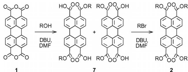
Scheme 2. Esterification of PTCDA with alkanol and alkyl halide in homogeneous solution (3 h at  $60^\circ\text{C}$  or 24 h at  $25^\circ\text{C}$ , yield  $>80\%$  for  $R = \text{ethyl, propyl, or butyl}$ ).
