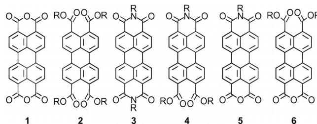
Scheme 1. PTCDA and its symmetrically and dissymmetrically substituted ester and carboxylic imide derivatives.
