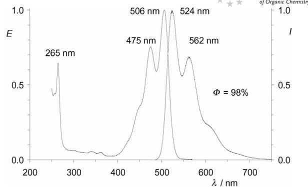
Figure 1. Absorption (left) and fluorescence (right) spectra of **4b** in chloroform.
