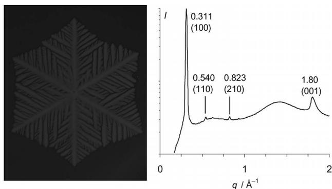
Figure 4. Left: homeotropic mesophase domain growing from the isotropic liquid between glass plates at cooling through the liquid to mesophase transition of **4c** (polarizing optical microscopy with slightly uncrossed polarizers, 0.5 mm × 0.6 mm). Right: powder X-ray diffraction spectrum of **4d** at room temperature (logarithmic intensity scaling). The indicated Miller indices correspond to a column lattice of hexagonal symmetry.
