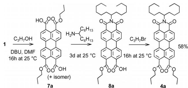
Scheme 3. One-pot formation of imido-diester in homogeneous solution by sequential addition of alcohol, alkylamine, and alkyl halide ( $R_f = 0.45$  in DCM on silica). Side products are the much less polar diimide [**3** with  $R = \text{CH}(\text{C}_6\text{H}_{13})_2$ ,  $R_f = 0.8$ ] and the much more polar tetraester (**2** with  $R = \text{C}_3\text{H}_7$ ,  $R_f = 0.23$ ). Yields are calculated with respect to the amine, using **1** in twofold excess.
