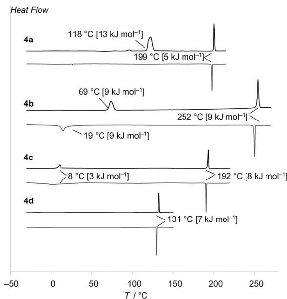
Figure 3. Differential calorimetry scans (heating in black, cooling in gray) of **4a–d** (5 K/min for **4a** and **4b**, 3 K/min for **4c** and **4d**). The temperatures given are onset temperatures. Transition enthalpies are given in brackets.
