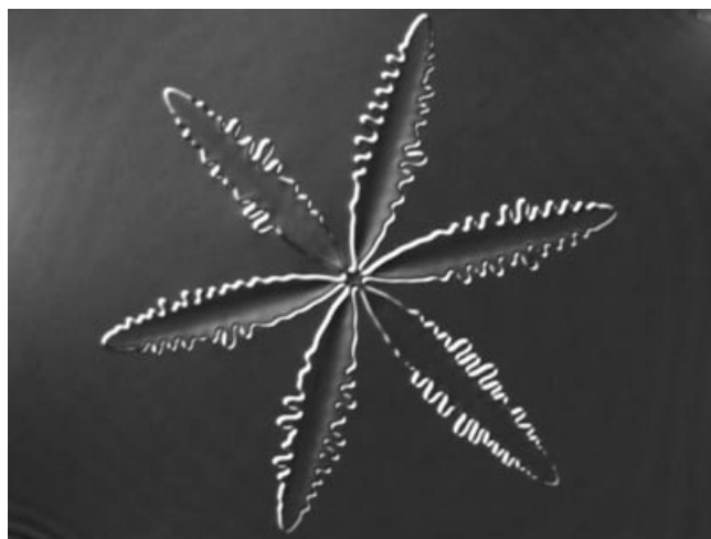
Figure 2. Growth of a hexagonal columnar liquid-crystalline domain in homeotropic orientation (columns perpendicular to substrate) of 6h upon cooling through the isotropic-to-LC phase-transition temperature on a silicon wafer, observed by differential interference contrast (DIC) microscopy in reflection (200 \mu\text{m} \times 150 \mu\text{m} ).
